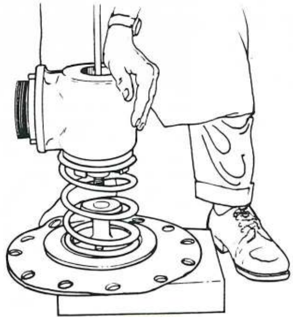
FIGURE 24 REMOVING ASSEMBLY BOLT
