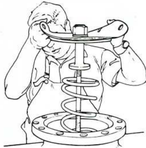
FIGURE 43 REMOVING RELIEF VALVE DIAPHRAGM ASSEMBLY
