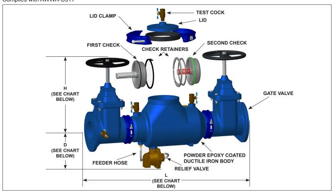
All RP devices must be installed where a drain is available to cover the discharge in event there is a backflow condition and the relief valve discharges. Discharge rates are as follows: ½" to 1" 5 GPM, 1 1/4" to 2" 20 GPM, 2 ½" to 6" 20 GPM, and 8" to 10" 60 GPM.
