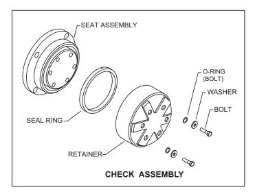
All Model 450 Double Check Valve Backflow Preventers must be inspected and maintained by licensed personnel at least once a year or more frequently as specified by local codes. Replacement of worn or damaged parts must only be made with genuine "ZURN WILKINS" parts.
