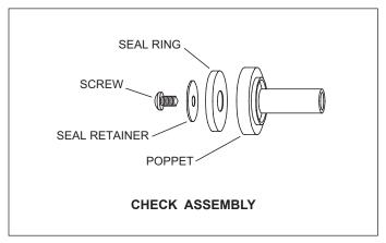
All Model 950XLTDA Double Check Detector Backflow Preventers must be inspected and maintained by licensed personnel at least once a year or more frequently as specified by local codes. Replacement of worn or damaged parts must only be made with genuine "ZURN WILKINS" parts.
