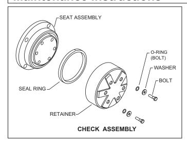
All Model 450ST Double Check Valve Backflow Preventers must be inspected and maintained by licensed personnel at least once a year or more frequently as specified by local codes. Replacement of worn or damaged parts must only be made with genuine "ZURN WILKINS" parts.
