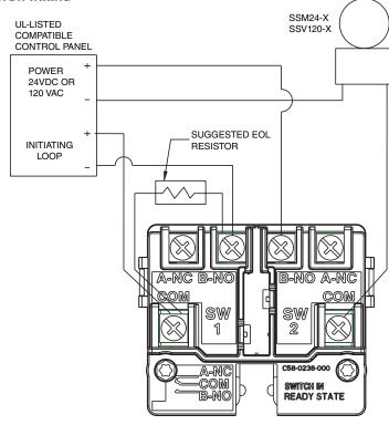
NOTE: COMMON AND B-NO CONNECTIONS WILL CLOSE WHEN VANE IS DEFECTED, I.E., WHEN WATER IS FLOWING. DUAL SWITCHES PERMIT APPLICATIONS TO BE COMBINED ON A SINGLE DETECTOR.
