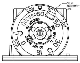
NOTE: RETARD TIME MAY EXCEED 90 SECONDS. ADJUST AND VERIFY THAT TIME DOES NOT EXCEED 90 SECONDS. NUMBER ON DIAL IS APPROXIMATE TIME DELAY IN SECONDS
